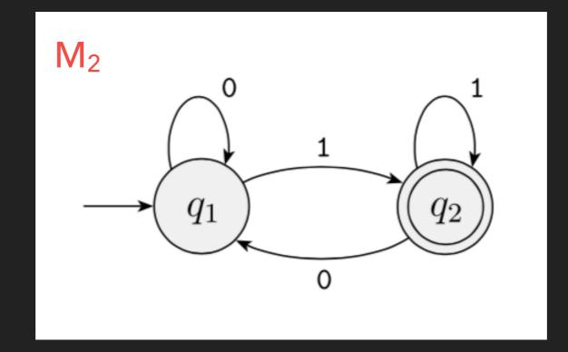
Defined by a 5-tuple:  $(Q, \Sigma, \delta, q_0, F)$   $M_2 = \{\{q_1, q_2\}, \{0, 1\}, \delta, q_1, \{q_2\}\}$   $\delta$  0 1  $q_1$   $q_1$   $q_2$  $q_2$   $q_1$   $q_2$
