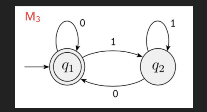
Defined by a 5-tuple:  $(Q, \Sigma, \delta, q_0, F)$  $M_3 = \{\{q_1, q_2\}, \{0, 1\}, \delta, q_1, \{q_1\}\} \begin{array}{c|c} \delta & 0 & 1 \\ \hline q_1 & q_1 & q_2 \\ \hline q_2 & q_1 & q_2 \end{array}$
